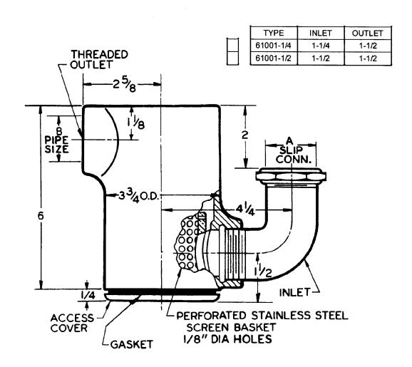
**NOTE:** 6" MIN. CLEARANCE REQUIRED BELOW COVER FOR REMOVABLE OF SEDIMENT BASKET.
